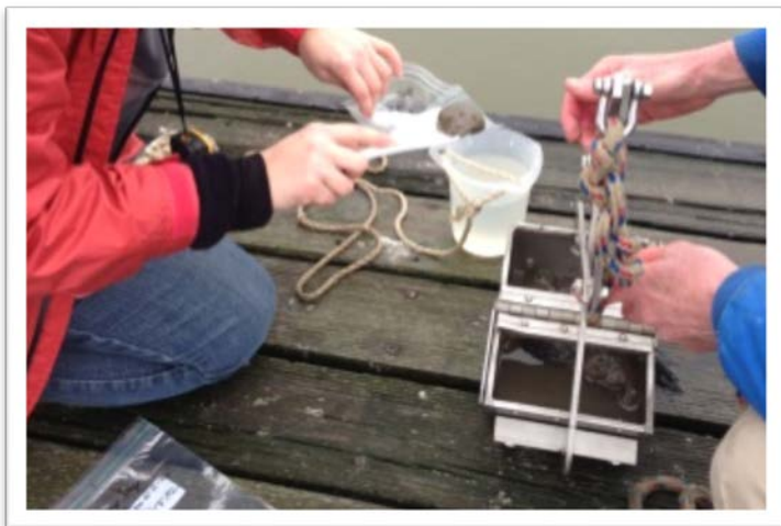
Figure 2. Sediment sampling using a Petite Ponar at Lake Erie marinas.
